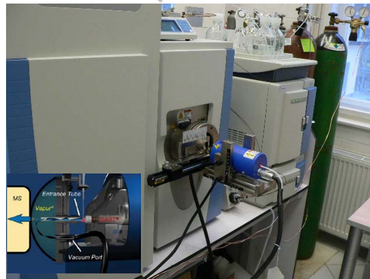
Exactive (Thermo Scientific) Orbitrap mass spectrometer ~ 10,000 – 100,000 fwhm
