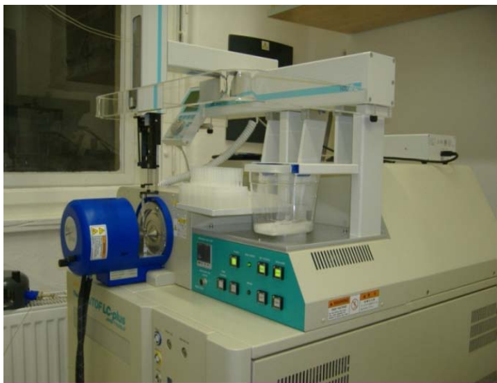
AccuTOF LP (Jeol) Time-of-flight mass spectrometer ~ 5000 – 7000 fwhm
